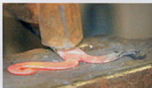
ABOVE: Red hot, just out of the forge, this iron door hinge exactly matches others in a restored mansion in Europe.
